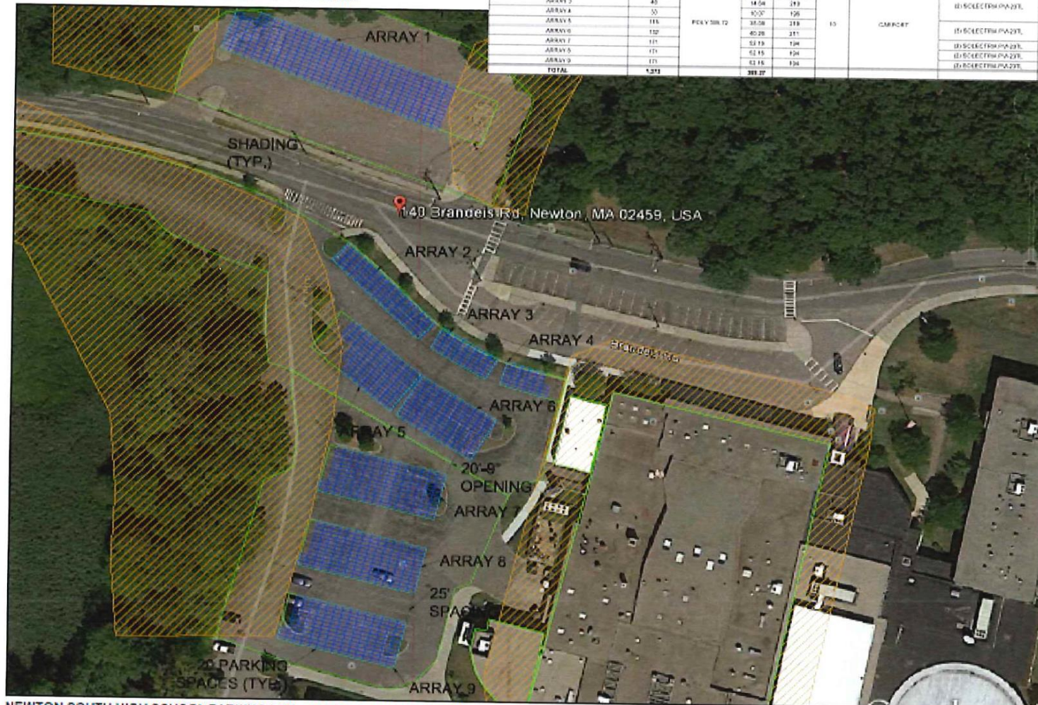
NEWTON SOUTH HIGH SCHOOL PARKING LOT - OVERALL ARRAY LAYOUT SCALE: 1" = 30'-0"
